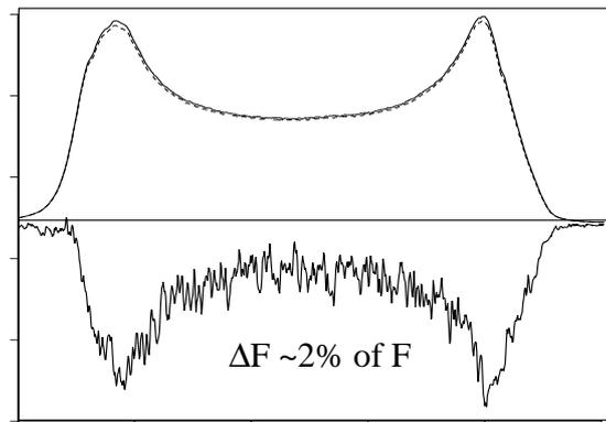
fig 2. total time (10 ps - 1.5 ns) integrated spectrum, upper panel: solid line no field over the sample, dashed with field. Lower panel: difference Field off minus field on.
